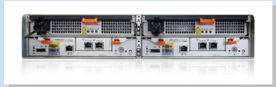
iSCSI Hardware Target EMC AX4-5i dual controller
